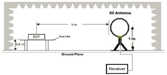
(2) Radiated Emission Test-Up Frequency 30MHz~1GHz
