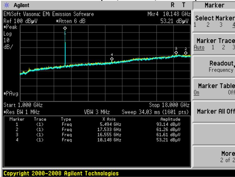
**Peak Radiated Transmitter Spurs, 5560 MHz, 6 to 54 Mbps**
