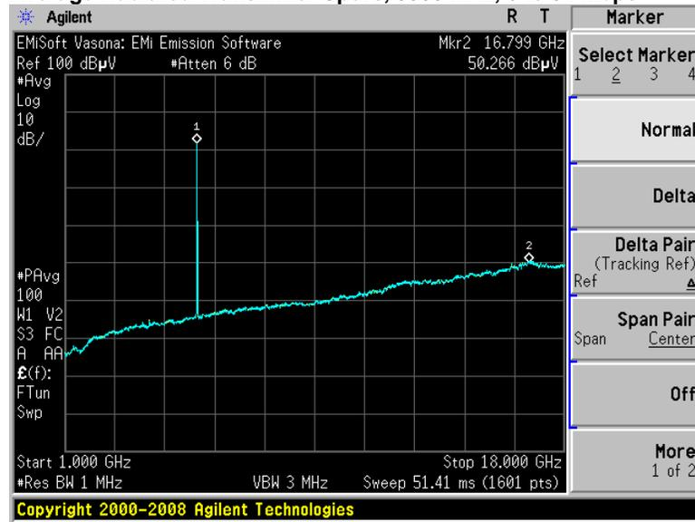
**Average Radiated Transmitter Spurs, 5560 MHz, 6 to 54 Mbps**
