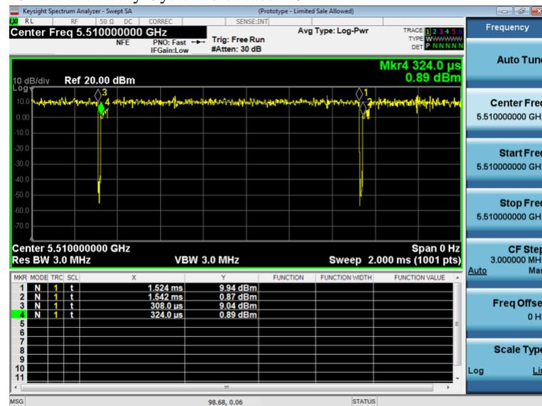
The Duty cycle of 40MHz BW is 98.7%, a 0.1dB CF is added to measurements.
