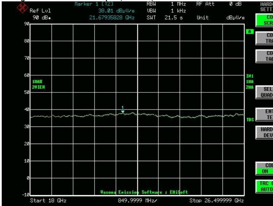
Average Radiated Transmitter Spurs, All rates, All Modes 18GHz to 26.5GHz
