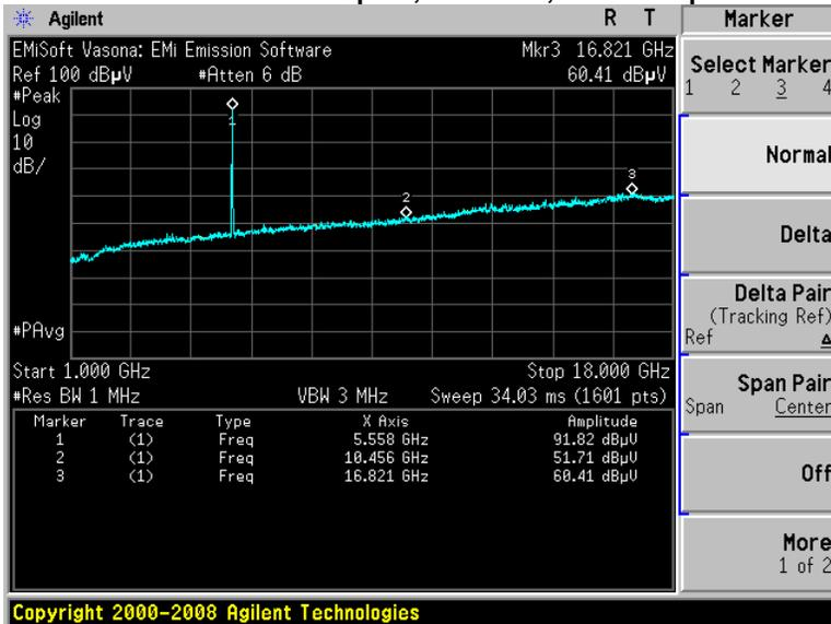
**Peak Radiated Transmitter Spurs, 5720 MHz, 6 to 54 Mbps**
