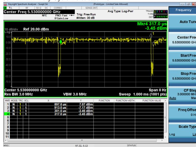
The Duty cycle of 80MHz BW is 97.3%, a 0.2dB CF is added to measurements.
