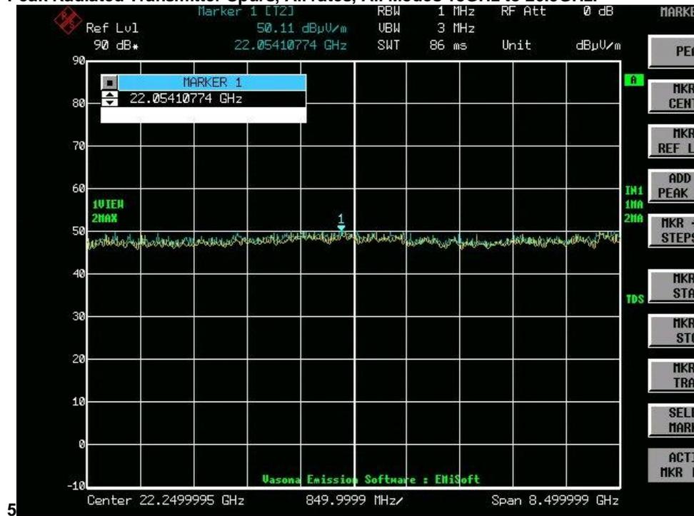
Peak Radiated Transmitter Spurs, All rates, All Modes 26.5GHz to 40GHz.
