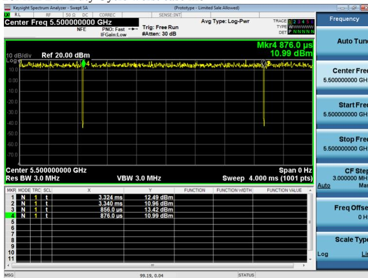
The Duty cycle is 99.2%, no correction is needed for measurements of 20MHz BW.
