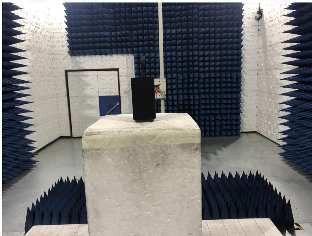
RADIATED EMISSION TEST SETUP ABOVE 1GHZ
