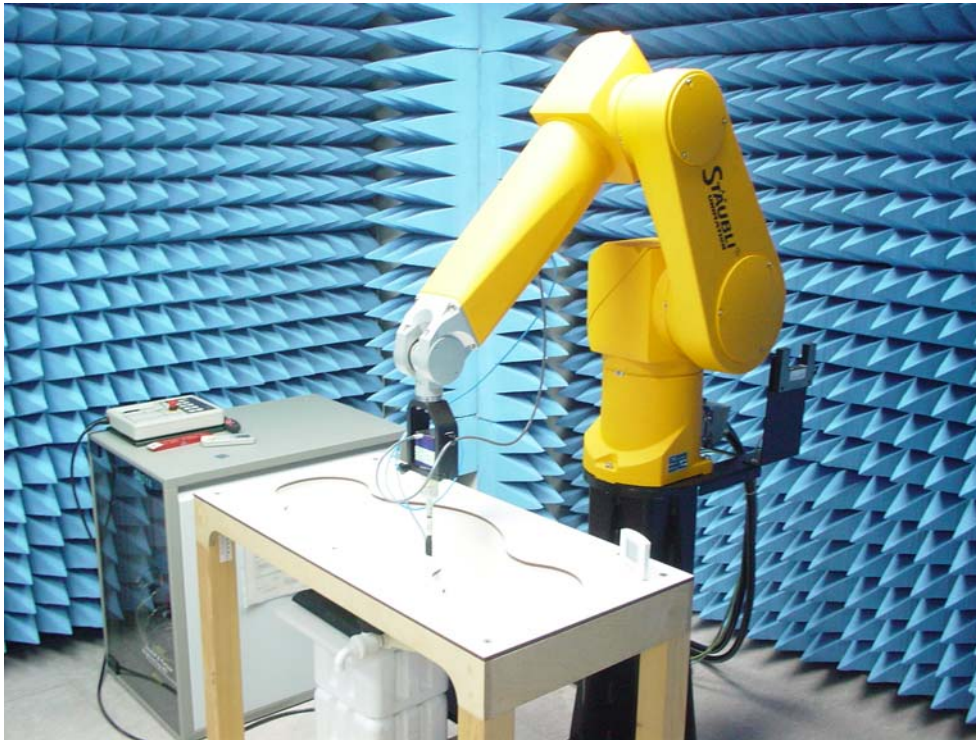
Fig.1 Photograph of the SAR measurement System
