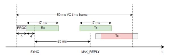
If we set the **MAX\_REPLY** time, measured from the SYNC event to **no larger than 20 ms**, then we have a buffer of 4 ms until the end of our VC time frame (5 + 4 + 20 + 17 - 50 = -4).
