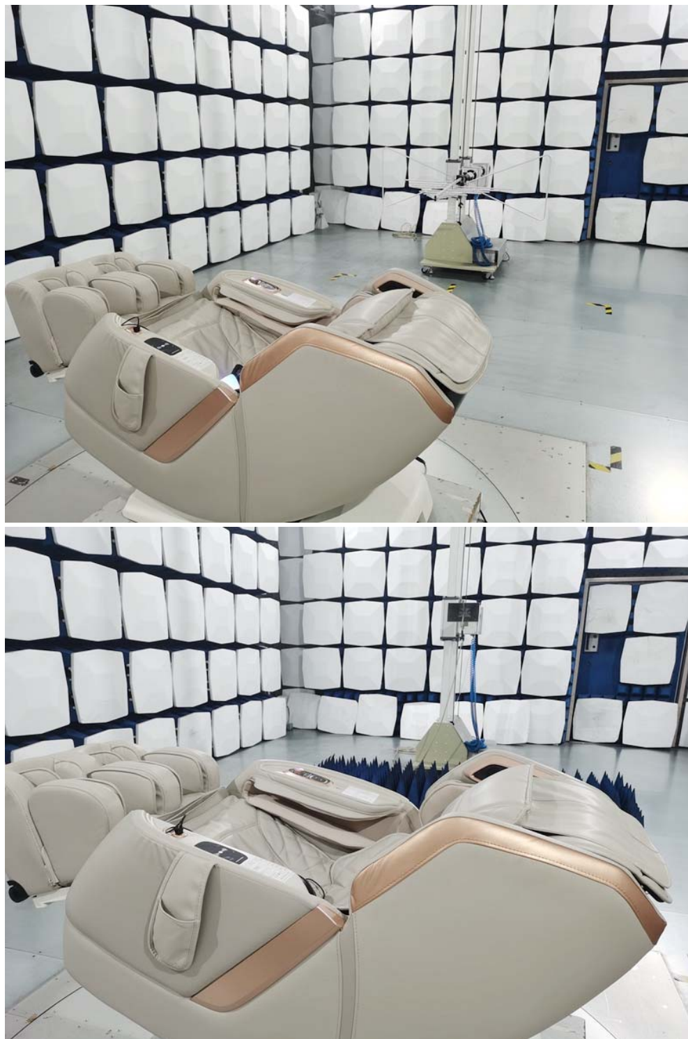
Radiated emission test view
