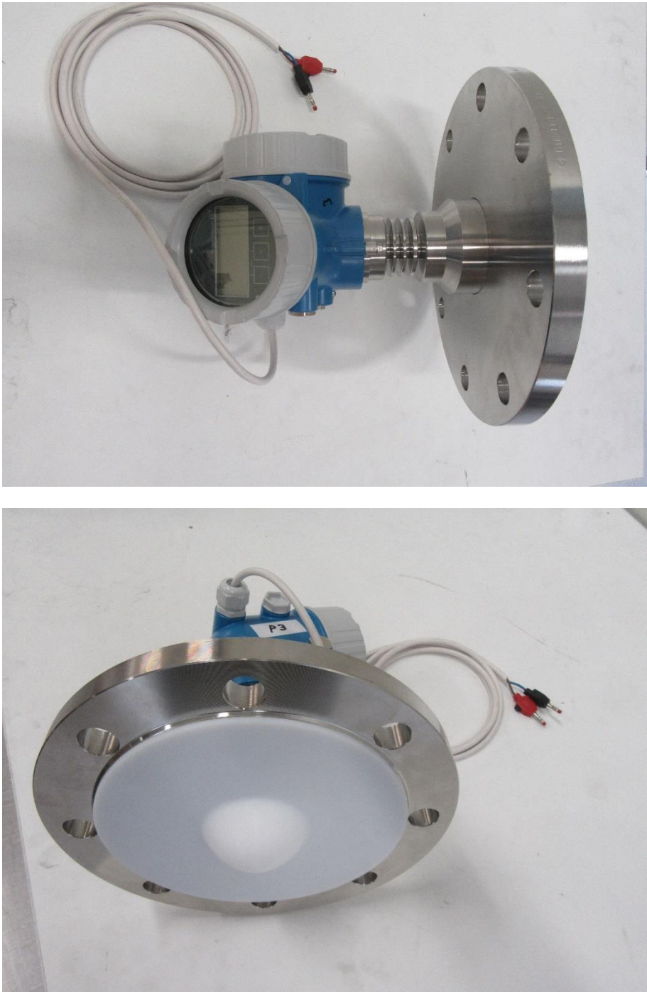
Figure 2 – EUT P3 (FMR51 with antenna Horn 40mm/1-1/2")
