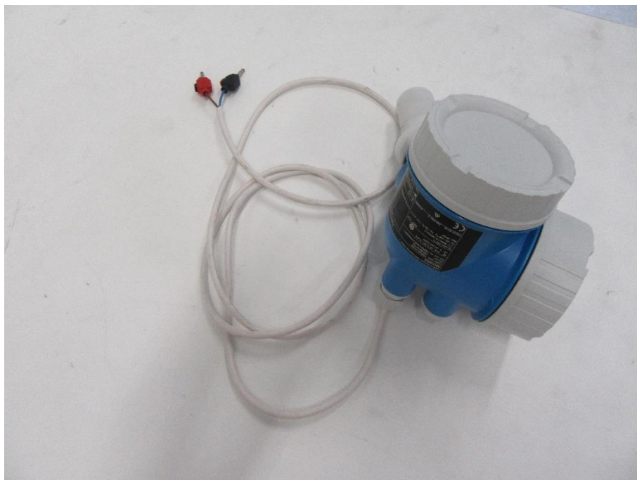
Figure 1 – EUT P1 (FMR50 with antenna Horn 40mm/1-1/2", PVDF encapsulated)
