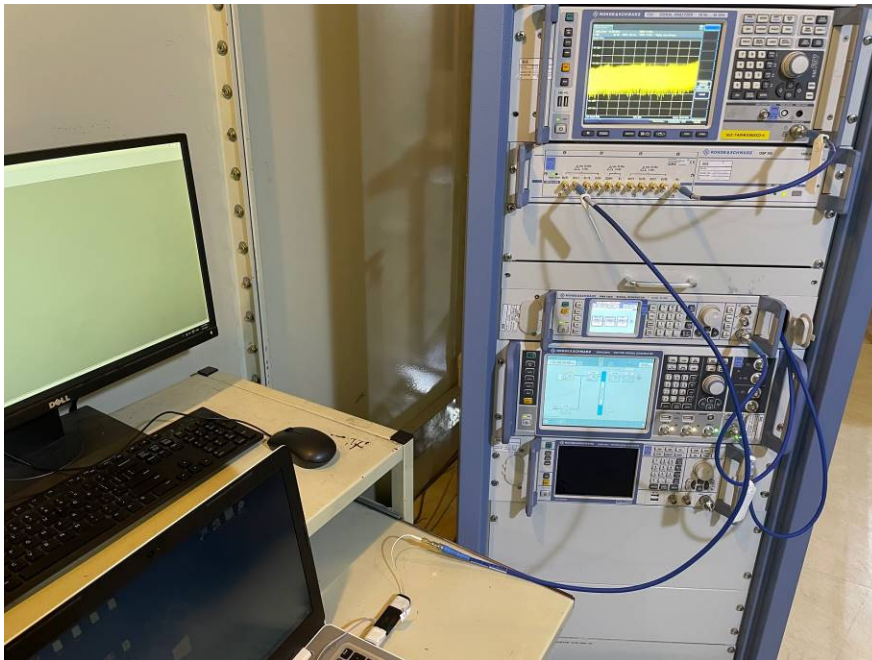
Conducted RF Power Test Setup
