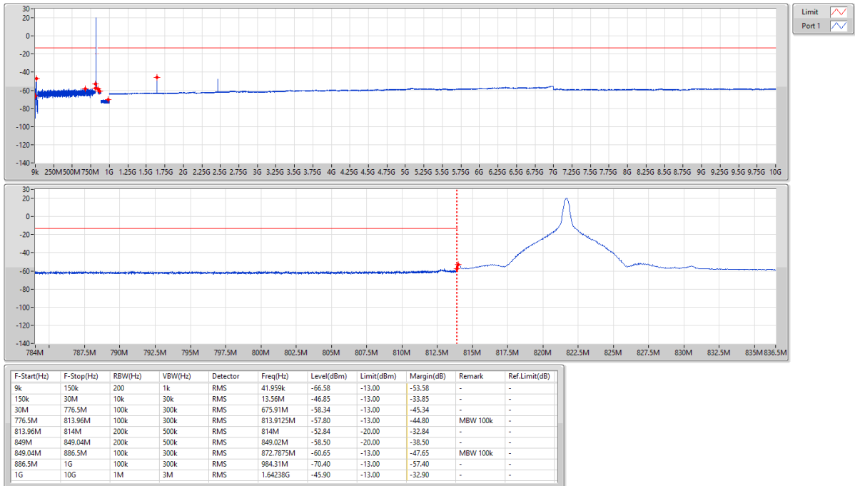
Band 26 LTE_15MHz_Nss1,64QAM_1TX 821.5MHz_64QAM_RB 1,#RB M
