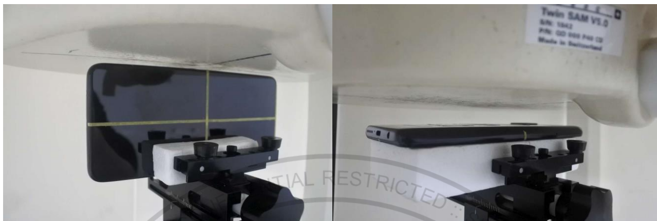
Left Side, Test Separation 3 mm(sensor off)
