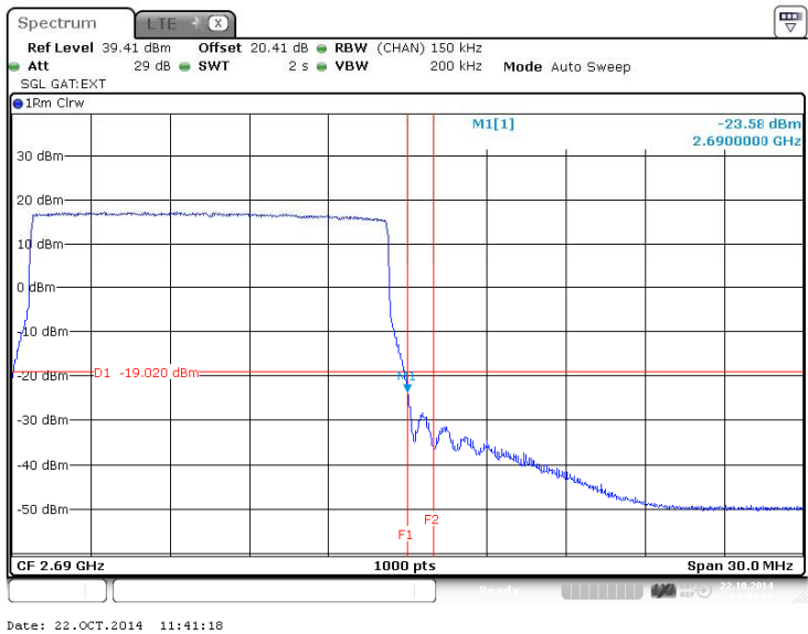
Figure 144 Spurious Emissions (Upper Band Edge) – QPSK (2682.5 MHz) (15MHz Channel BW)
