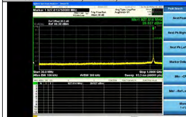
Modulation: 2FSK, Mode 66, 927.6MHz (30Hz-1GHz)
