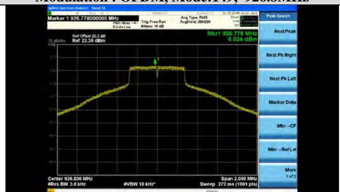
Modulation : OFDM , Mode:149, 926.8MHz
