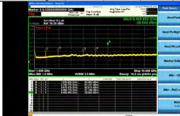
Mod: OQPSK, Mode 192, 927.8MHz (1-10GHz) Peak
