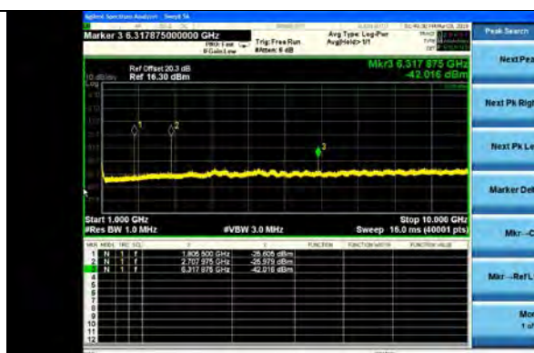
Modulation: 2FSK, Mode 66, 915.2MHz (1-10GHz)
