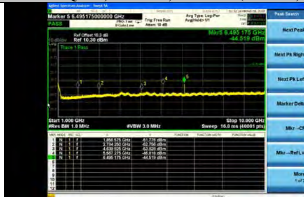
Mod: OQPSK, Mode 192, 927.8MHz (1-10GHz) Peak
