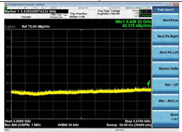
802.11a | Channel 144 | 6 Mbps | Y Plane 4000-5470 MHz | Horizontal
