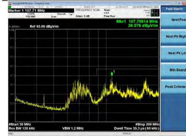
802.11a | Channel 165 | 6 Mbps | Y Plane 30-200 MHz | Horizontal
