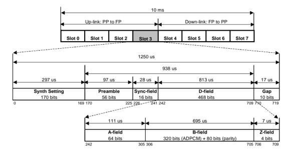
The EDCT TDMA frame structure is shown below:
