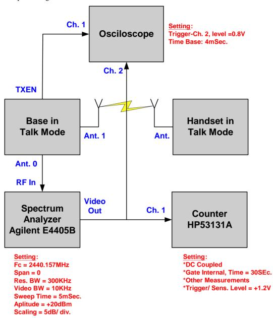
Step 1: Establish Single Channel "Talk mode" BS/HS Link on Ch55. Note SA Video output level on Scope for both Antenna Selections. Repeat for Adjacent Channels – See Plot 7. Note that a "pulse threshold" = 1.2V clearly indicates a Ch55 "hit".
