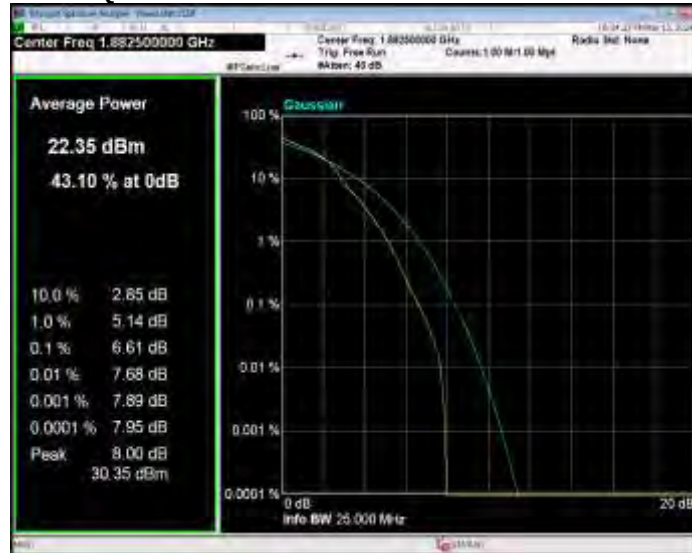
Band25 16QAM BW=20MHz Channel=26590 RB Size=1 Position=#0
