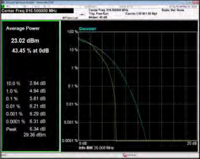
Band26(814-824) 16QAM BW=5MHz Channel=26740 RB Size=1 Position=#0
