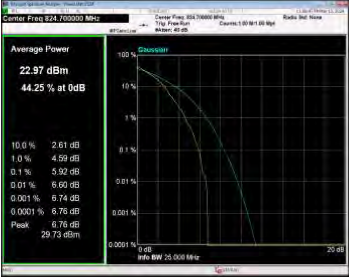
Band26(824-849) QPSK BW=1.4MHz Channel=26797 RB Size=1 Position=#0
