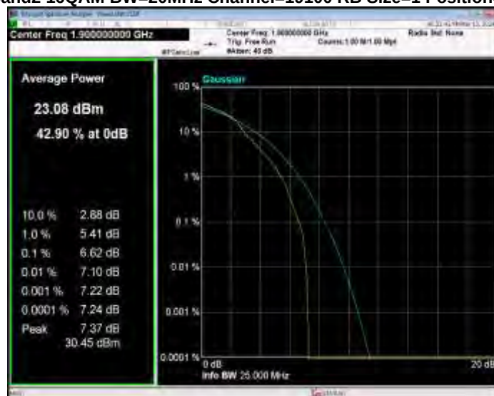
Band2 16QAM BW=20MHz Channel=19100 RB Size=1 Position=#0
