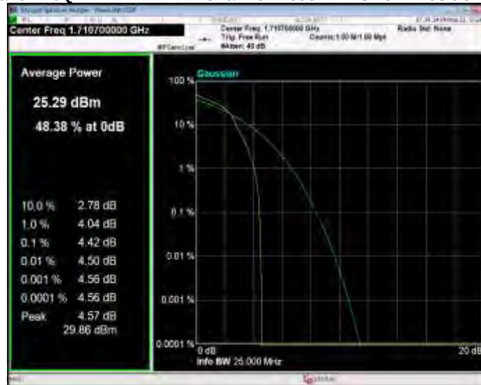
Band4 16QAM BW=1.4MHz Channel=20175 RB Size=1 Position=#0
