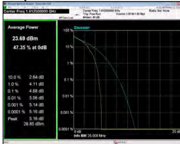
Band25 QPSK BW=5MHz Channel=26665 RB Size=1 Position=#0
