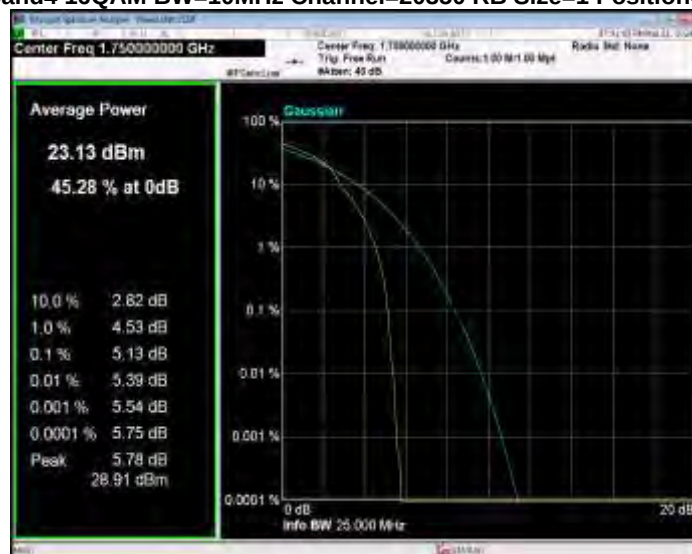
Band4 16QAM BW=10MHz Channel=20350 RB Size=1 Position=#0
