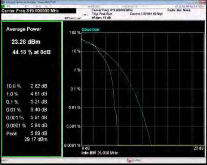
Band26(814-824) 16QAM BW=5MHz Channel=26740 RB Size=1 Position=#0
