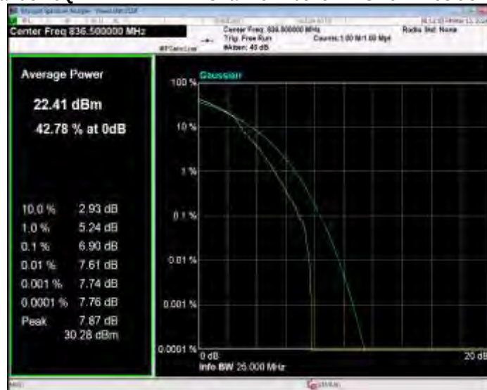
Band5 16QAM BW=1.4MHz Channel=20643 RB Size=1 Position=#0
