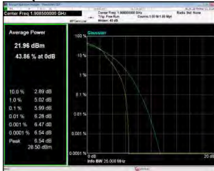
Band2 16QAM BW=3MHz Channel=19185 RB Size=1 Position=#0
