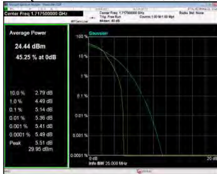
Band4 16QAM BW=15MHz Channel=20175 RB Size=1 Position=#0
