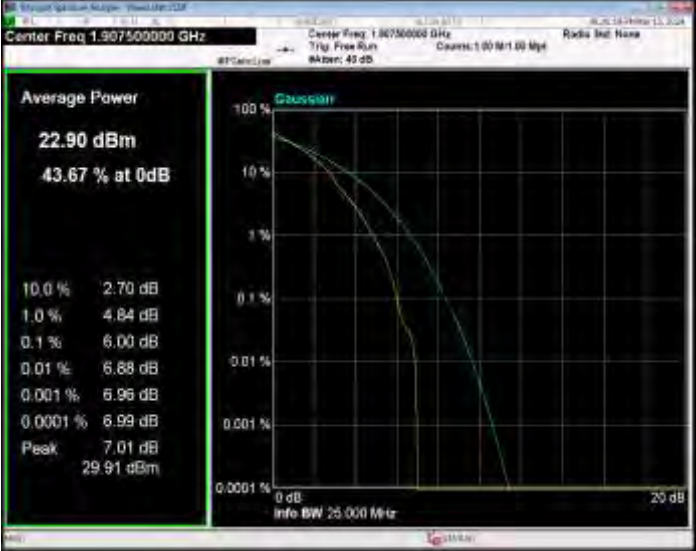
Band2 QPSK BW=5MHz Channel=19175 RB Size=1 Position=#0
