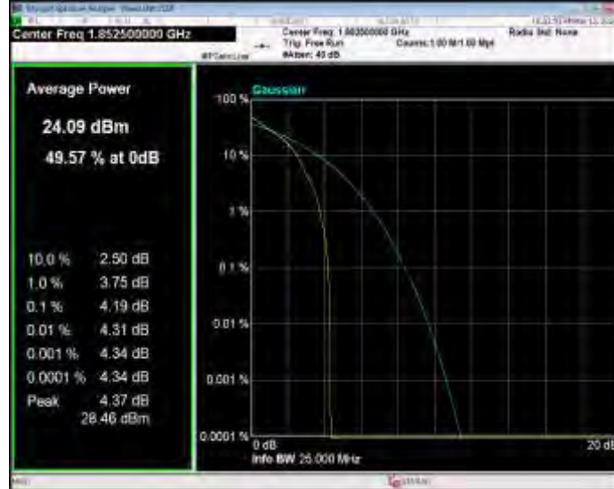
Band25 QPSK BW=5MHz Channel=26365 RB Size=1 Position=#0
