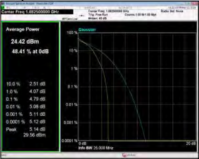
Band25 QPSK BW=1.4MHz Channel=26683 RB Size=1 Position=#0
