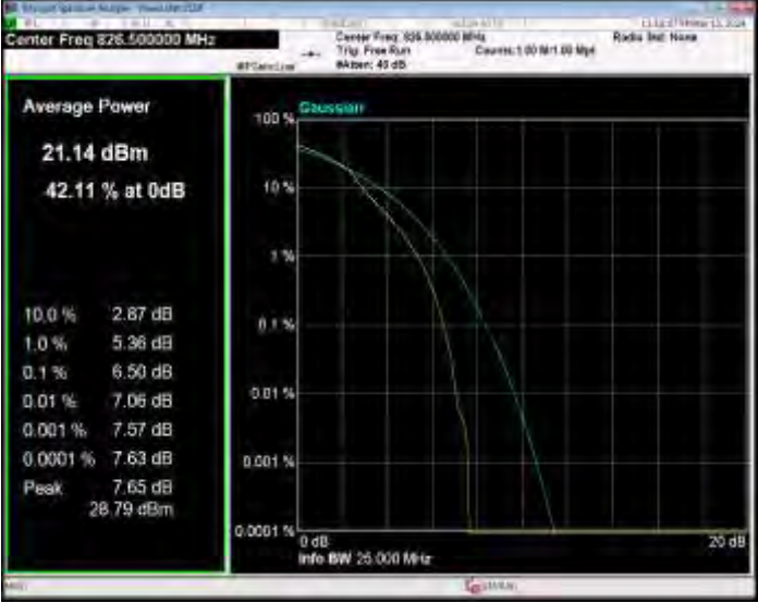
Band26(824-849) 16QAM BW=5MHz Channel=26815 RB Size=1 Position=#0
