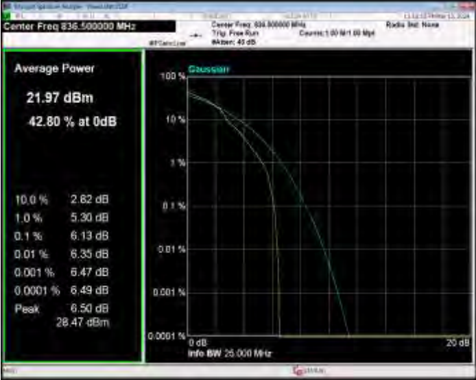
Band26(824-849) 16QAM BW=5MHz Channel=27015 RB Size=1 Position=#0
