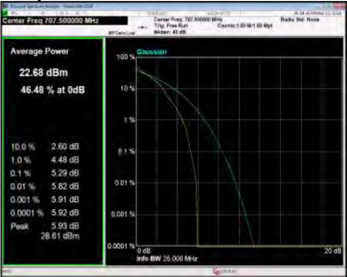
Band12 QPSK BW=1.4MHz Channel=23173 RB Size=1 Position=#0
