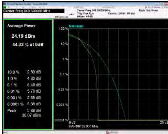
Band5 16QAM BW=1.4MHz Channel=20643 RB Size=1 Position=#0
