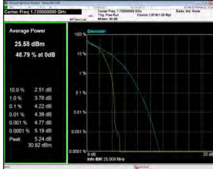
Band4 QPSK BW=20MHz Channel=20175 RB Size=1 Position=#0
