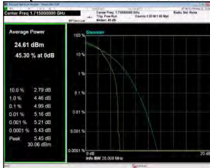
Band4 16QAM BW=10MHz Channel=20175 RB Size=1 Position=#0
