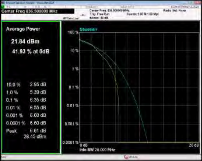
Band26(824-849) 16QAM BW=3MHz Channel=27025 RB Size=1 Position=#0
