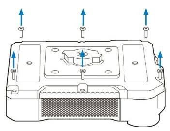
3 Remove the back of the camera.
