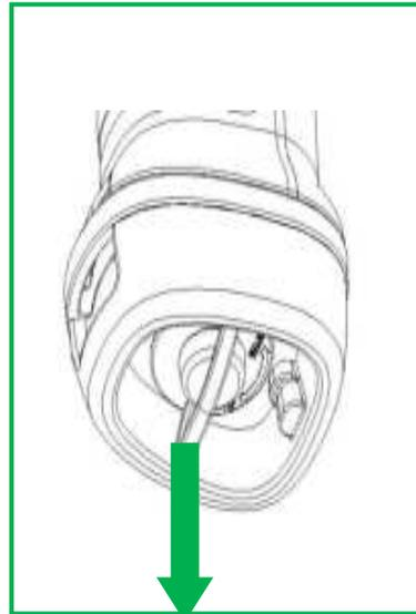
Battery Removal Steps: Pull out the switch ring on the battery and turn it counterclockwise about 45° to unlock the battery, then pull out the battery in the direction shown in the picture.
