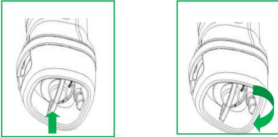
Battery Installation Steps: Insert the battery in the direction as shown, then turn it clockwise about 45° to lock the battery, and finally return the switch ring to its place.
