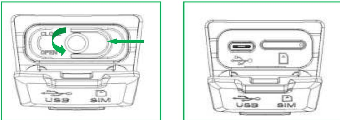
USB charging steps: pull out the switch ring in the direction as shown in the picture, unlock the interface cover by rotating counterclockwise about 45°, pull out the interface cover vertically to reveal the USB port, connect the USB charger or computer. If charging on, observe the screen power display, charge to 100%, stop charging. If the power off charging, observe the indicator light, flashing red light for charging status, flashing green light is fully charged. Disconnect the USB after
