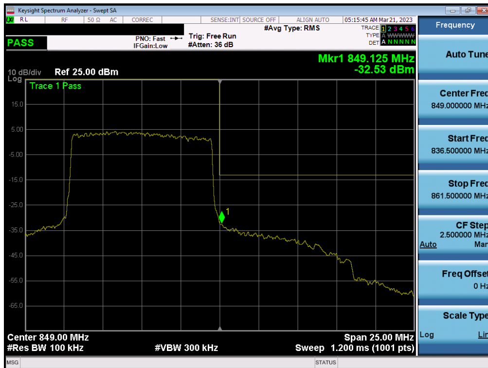
Plot 7-19. Upper Band Edge Plot (LTE Band 5 - 10MHz QPSK – Full RB)
