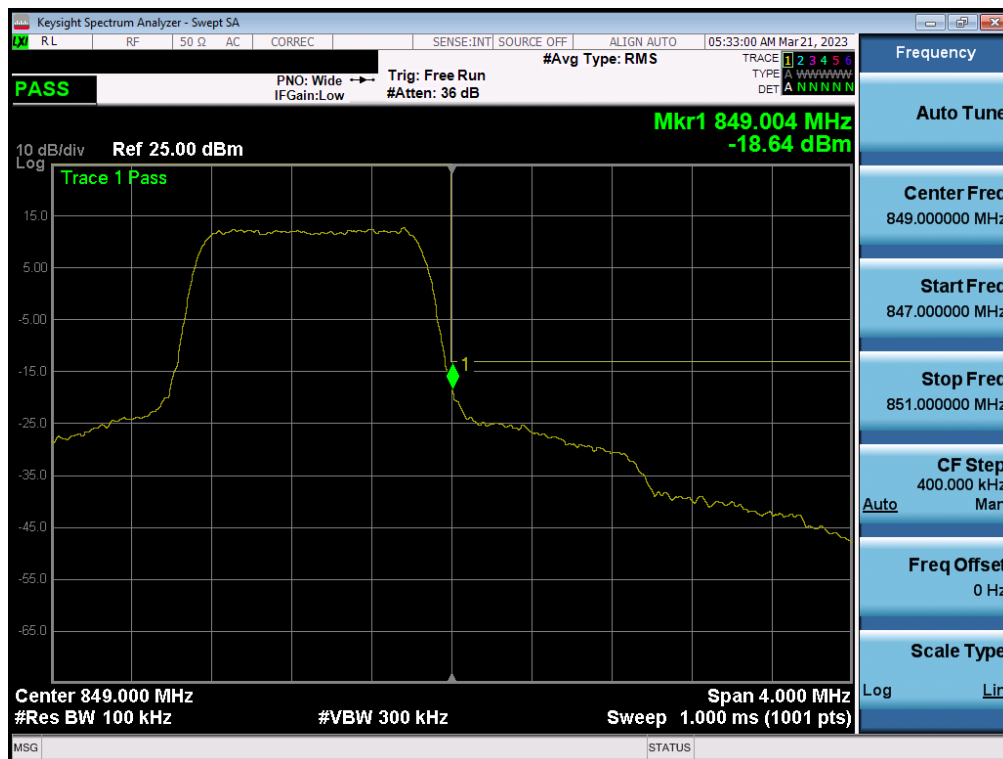
Plot 7-25. Upper Band Edge Plot (LTE Band 5 – 1.4MHz QPSK – Full RB)
