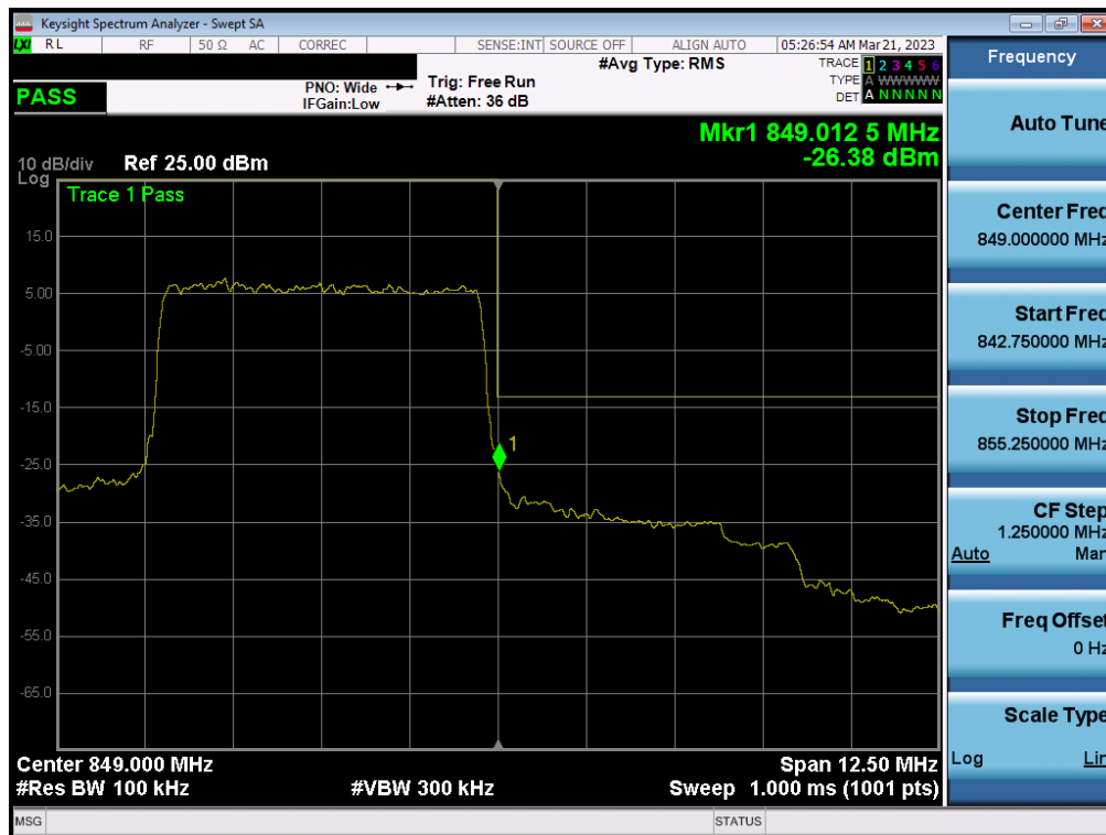
Plot 7-21. Upper Band Edge Plot (LTE Band 5 - 5MHz QPSK – Full RB)
