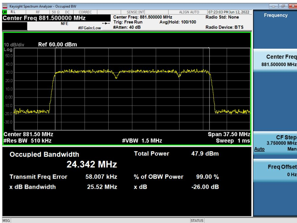
**Antenna 3 / B5 DSS 10 MHz 1 Carrier + 5G NR n5 10 MHz 1 Carrier + LTE B5 5 MHz 1 Carrier [3 Carrier] / Contiguous / 16QAM / Middle**
