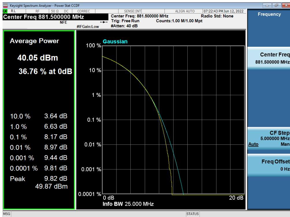
**Antenna 3 / B5 DSS 10 MHz 1 Carrier + 5G NR n5 10 MHz 1 Carrier + LTE B5 5 MHz 1 Carrier [3 Carrier] / Contiguous / 16QAM / Middle**
