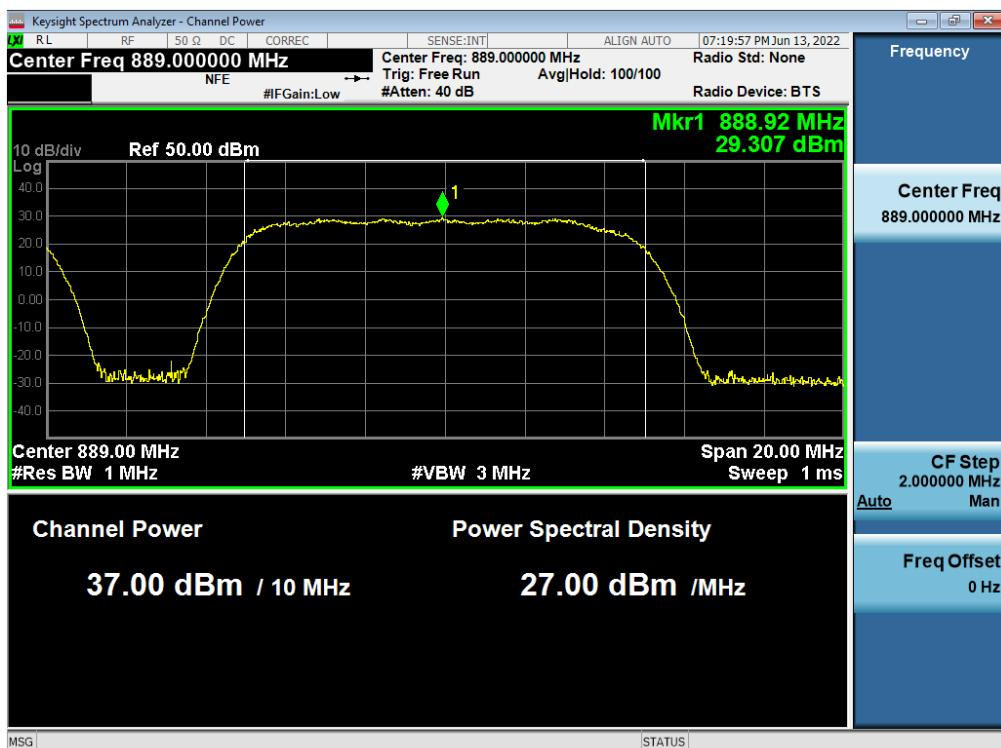
**Antenna 0 / 5G NR n5 5 MHz 1 Carrier + (LTE B5 5 MHz 1 Carrier + B5 DSS 10 MHz 1 Carrier) [3 Carrier] (1C+2C) / Non-Contiguous / 5G NR n5 5 MHz / 16QAM / Low**
