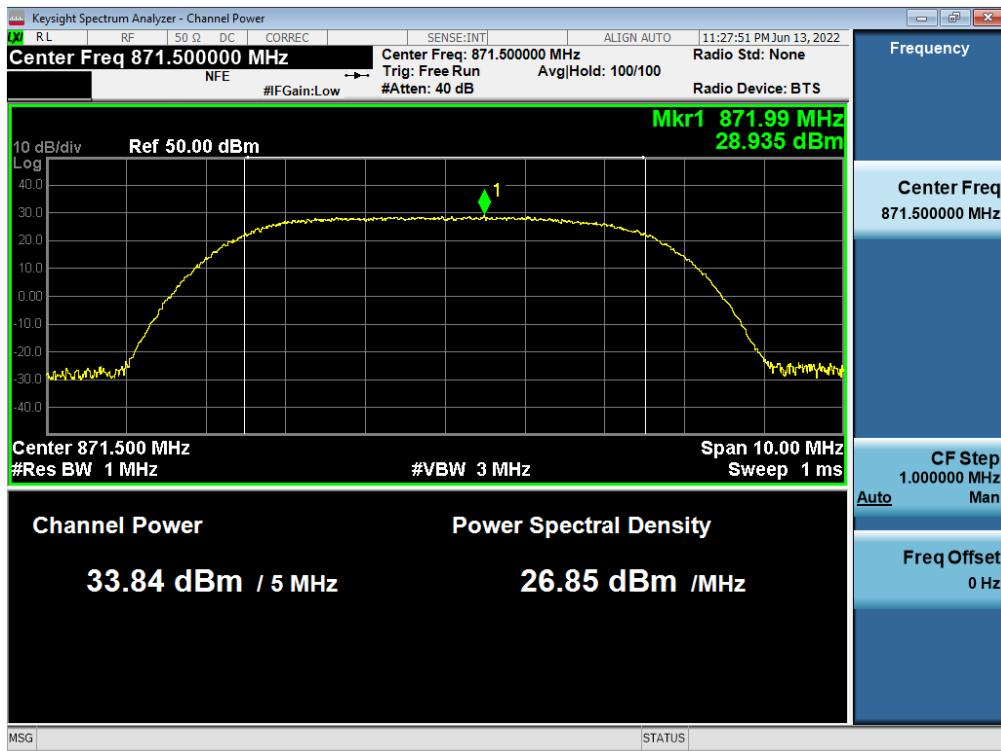
**Antenna 0 / 5G NR n5 5 MHz 1 Carrier + (LTE B5 5 MHz 1 Carrier + B5 DSS 10 MHz 1 Carrier) [3 Carrier] (1C+2C) / Non-Contiguous / LTE B5 5 MHz + B5 DSS 10 MHz / 16QAM / High**
