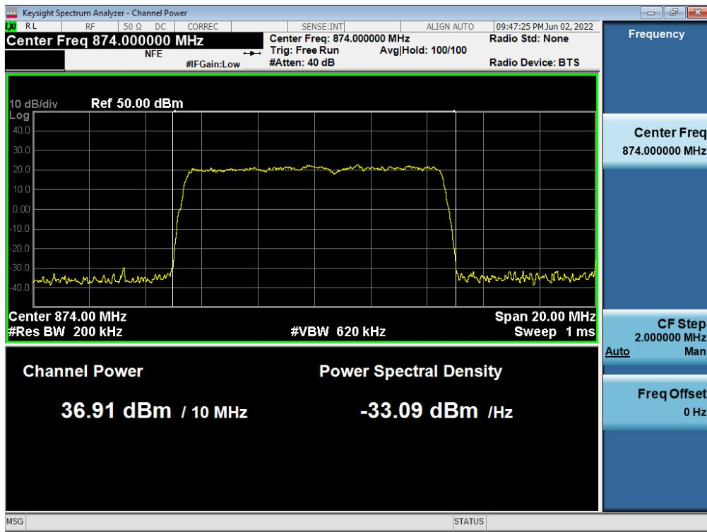
**Antenna 3 / B5 DSS 10 MHz 1 Carrier + B5 DSS 10 MHz 1 Carrier [2 Carrier] / Non-Contiguous / B5 DSS 10 MHz / 16QAM / High**
