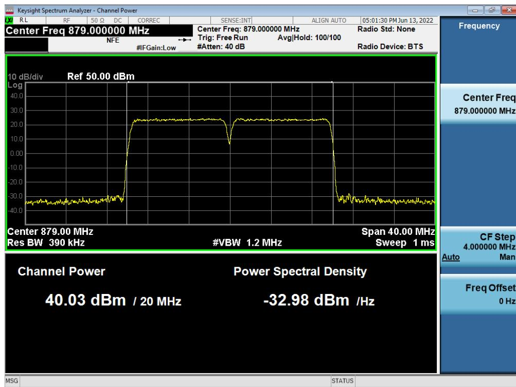
**Antenna 3 / B5 DSS 10 MHz 1 Carrier + 5G NR n5 5 MHz 1 Carrier + LTE B5 5 MHz 1 Carrier [3 Carrier] / Contiguous / 64QAM / High**
