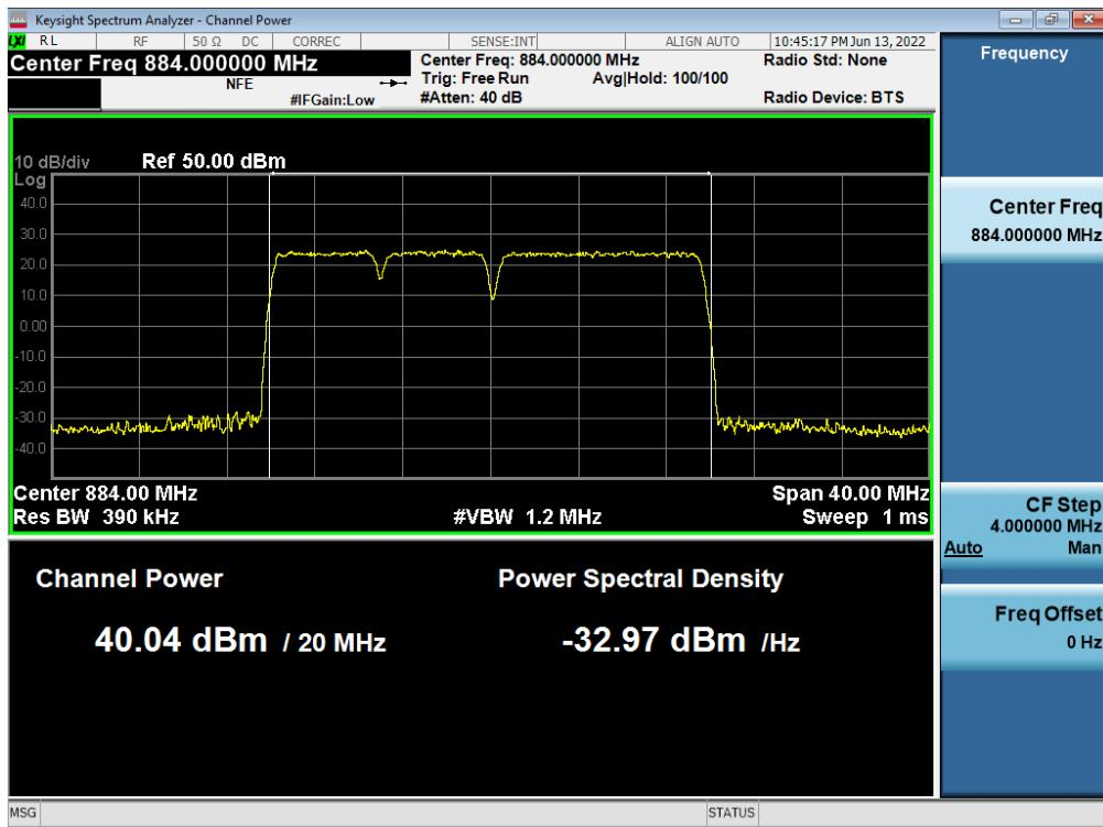
**Antenna 3 / 5G NR n5 10 MHz 1 Carrier + 5G NR n5 10 MHz 1 Carrier + LTE B5 5 MHz 1 Carrier [3 Carrier] / Contiguous / 256QAM / Middle**
