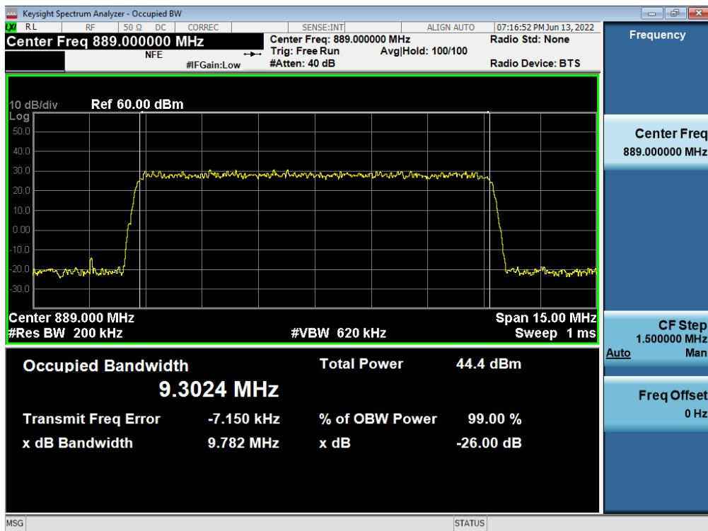
**Antenna 0 / 5G NR n5 5 MHz 1 Carrier + (LTE B5 5 MHz 1 Carrier + B5 DSS 10 MHz 1 Carrier) [3 Carrier] (1C+2C) / Non-Contiguous / 5G NR n5 5 MHz / QPSK / Low**
