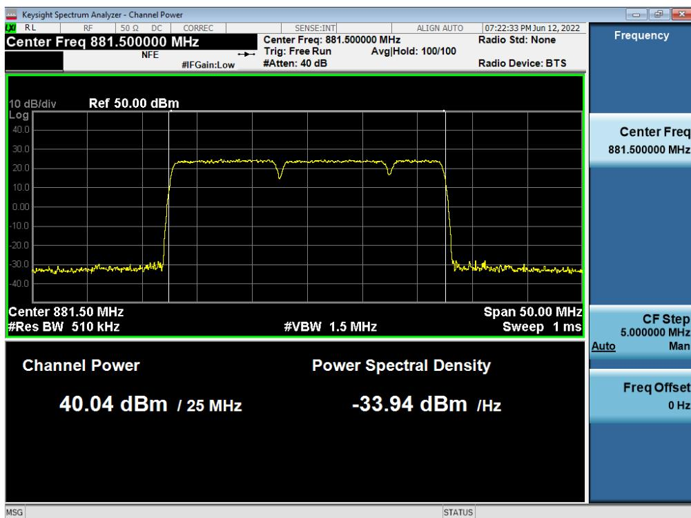
**Antenna 3 / B5 DSS 10 MHz 1 Carrier + 5G NR n5 10 MHz 1 Carrier + LTE B5 5 MHz 1 Carrier [3 Carrier] / Contiguous / 16QAM / Middle**
