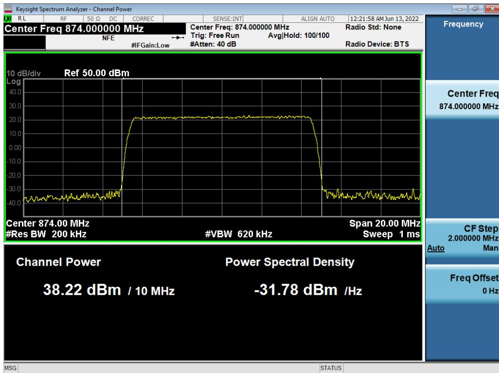
**Antenna 3 / B5 DSS 10 MHz 1 Carrier + 5G NR n5 5 MHz 1 Carrier [2 Carrier] / Non-Contiguous / 5G NR n5 5 MHz / QPSK / High**
