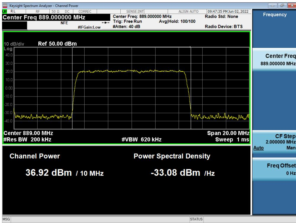
**Antenna 1 / 5G NR n5 5 MHz 1 Carrier + 5G NR n5 5 MHz 1 Carrier [2 Carrier] / Non-Contiguous / 5G NR n5 5 MHz / 16QAM / Low**
