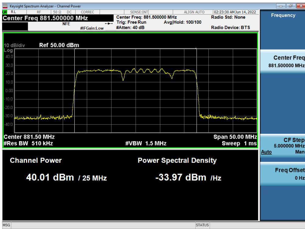
**Antenna 3 / B5 DSS 10 MHz 1 Carrier + B5 DSS 10 MHz 1 Carrier [2 Carrier] / Non-Contiguous / B5 DSS 10 MHz / 16QAM / Low**
