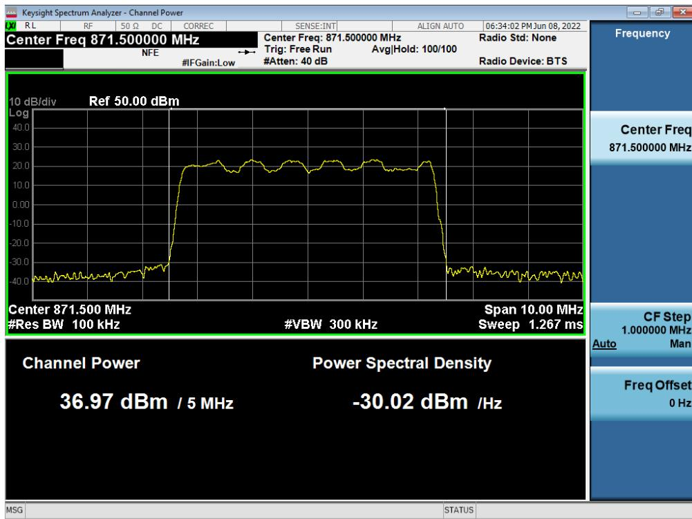
**Antenna 1 / 5G NR n5 5 MHz 1 Carrier + 5G NR n5 5 MHz 1 Carrier [2 Carrier] / Non-Contiguous / 5G NR n5 5 MHz / 16QAM / High**
