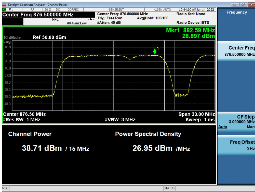
**Antenna 3 / (B5 DSS 10 MHz 1 Carrier + LTE B5 5 MHz 1 Carrier) + 5G NR n5 5 MHz 1 Carrier [3 Carrier] (2C+1C) / Non-Contiguous / 5G NR n5 5 MHz / 16QAM / High**
