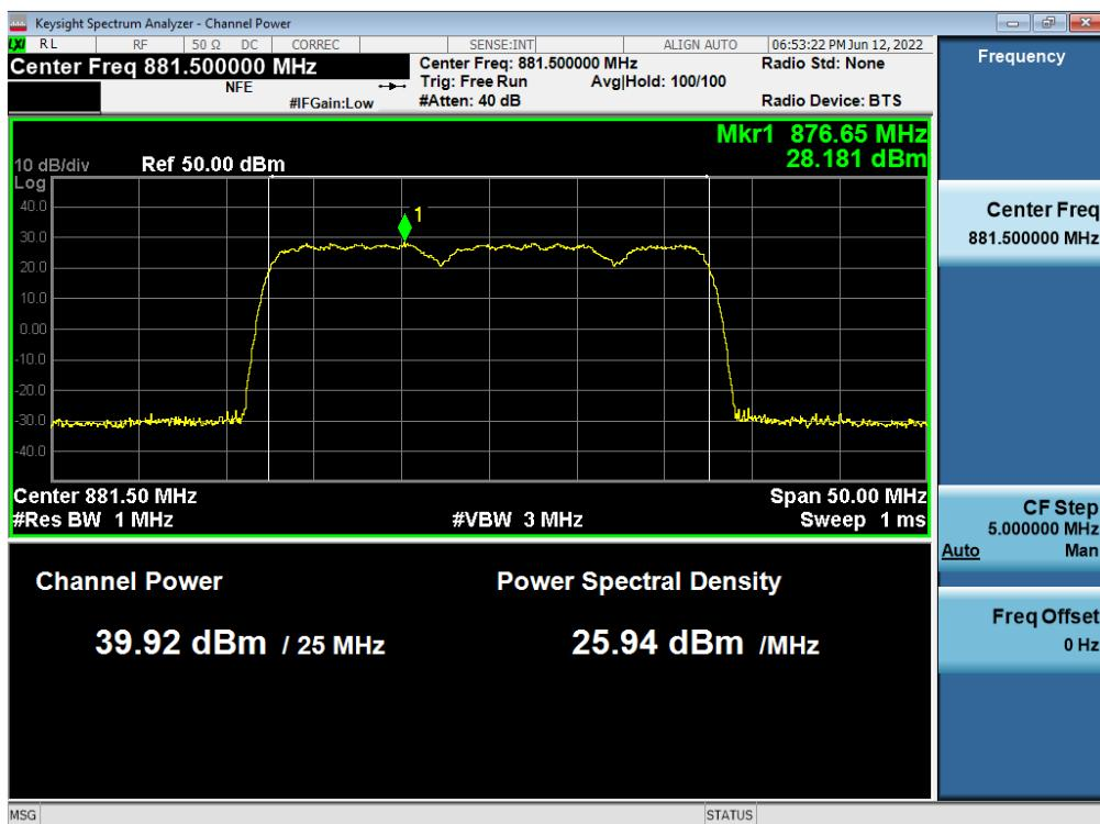
**Antenna 2 / B5 DSS 10 MHz 1 Carrier + 5G NR n5 10 MHz 1 Carrier + LTE B5 5 MHz 1 Carrier [3 Carrier] / Contiguous / 16QAM / Middle**
