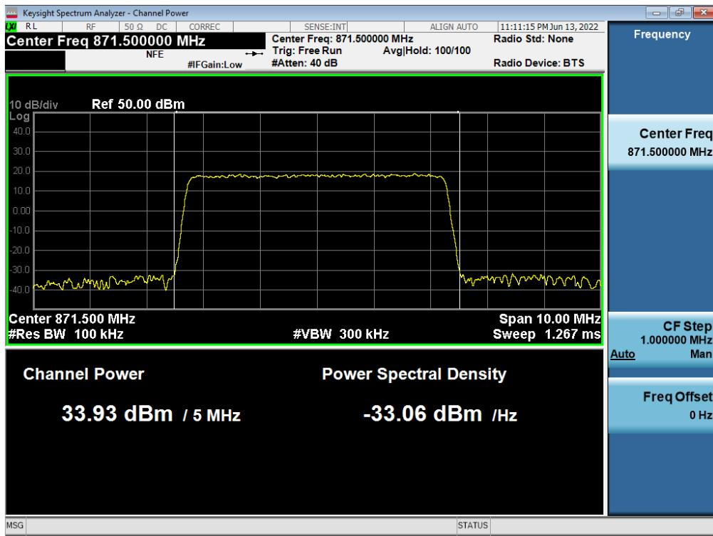
**Antenna 0 / 5G NR n5 5 MHz 1 Carrier + (LTE B5 5 MHz 1 Carrier + B5 DSS 10 MHz 1 Carrier) [3 Carrier] (1C+2C) / Non-Contiguous / LTE B5 5 MHz + B5 DSS 10 MHz / QPSK / High**
