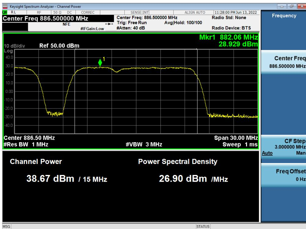
**Antenna 3 / (B5 DSS 10 MHz 1 Carrier + LTE B5 5 MHz 1 Carrier) + 5G NR n5 5 MHz 1 Carrier [3 Carrier] (2C+1C) / Non-Contiguous / B5 DSS 10 MHz + LTE B5 5 MHz / 16QAM / Low**
