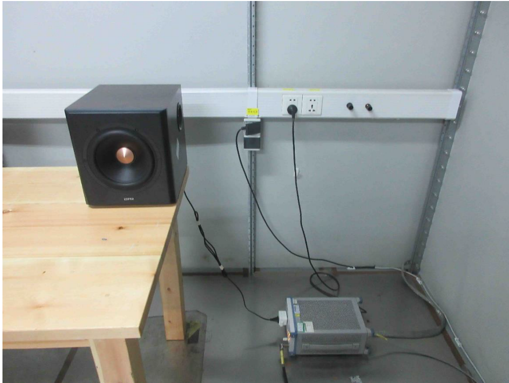
Photograph 1: Set-up for Conducted Emission on AC Mains
