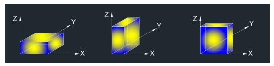
Note: For all radiated test, EUT in each of three orthogonal axis emissions had been tested, but only the worst case (X axis) data recorded in the report.
