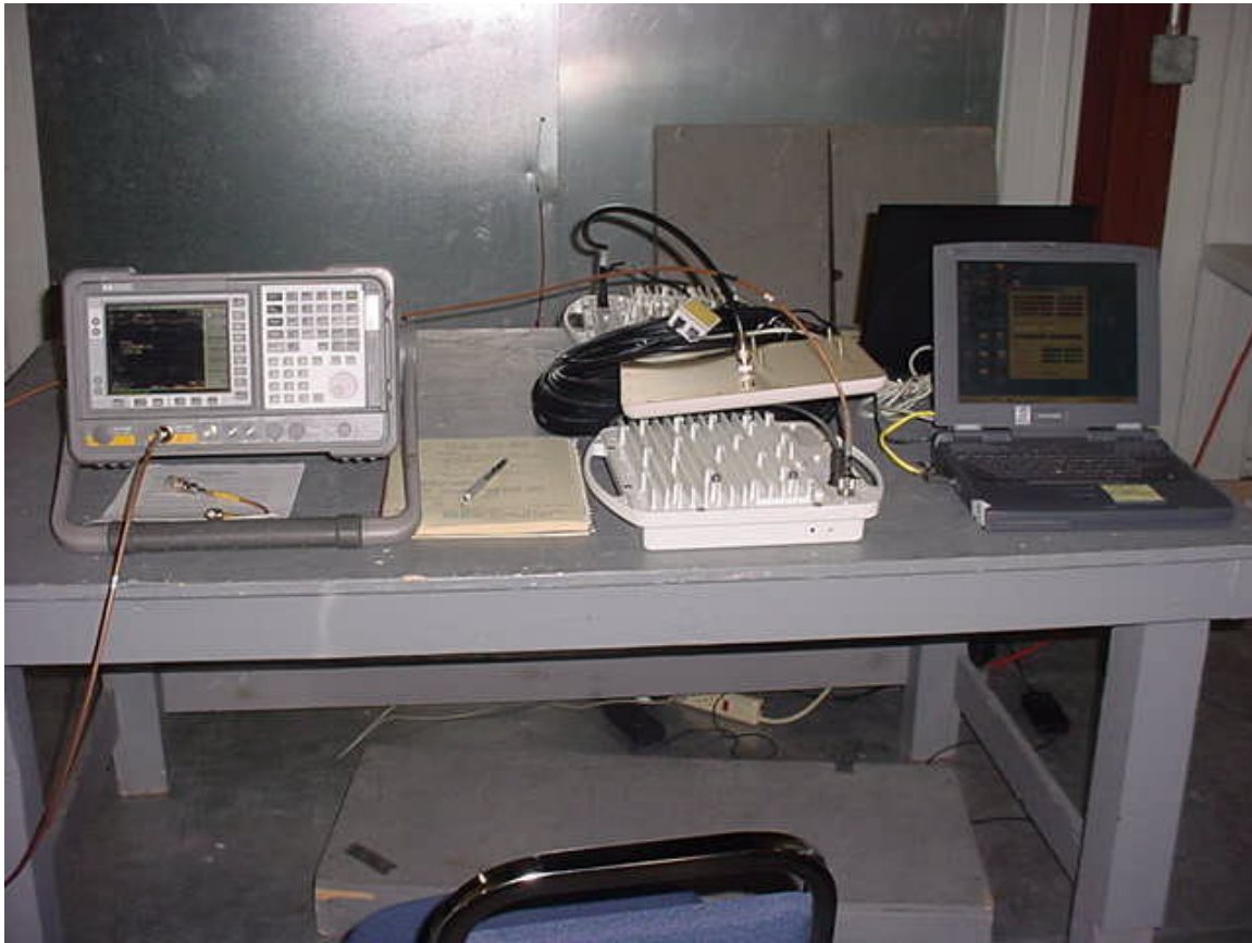
Antenna Port Conducted Measurements
