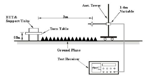
The radiated emission tests were performed in the 3 meters, using the setup accordance with the ANSI C63.10-2013. The specification used was the FCC 15.209 and FCC 15.319 (g) limits.
