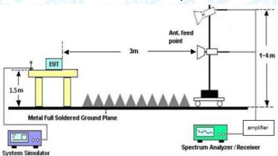
**Above 1GHz Test Setup**
