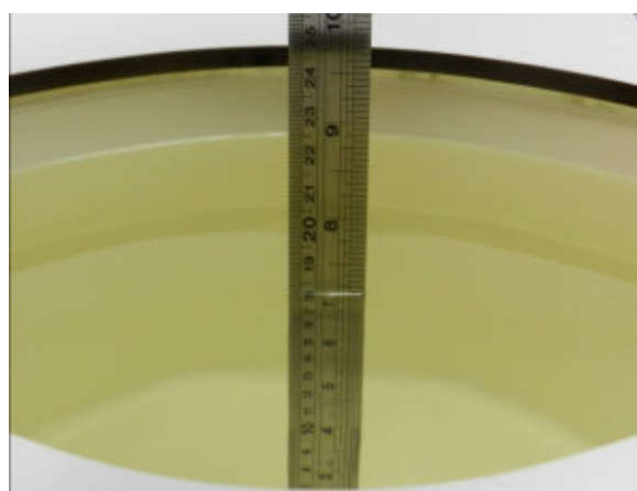
Fig 11.2 Photo of Liquid Height for Body SAR
