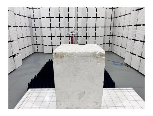
Set-up for Radiated Spurious Emission, Above 1GHz
