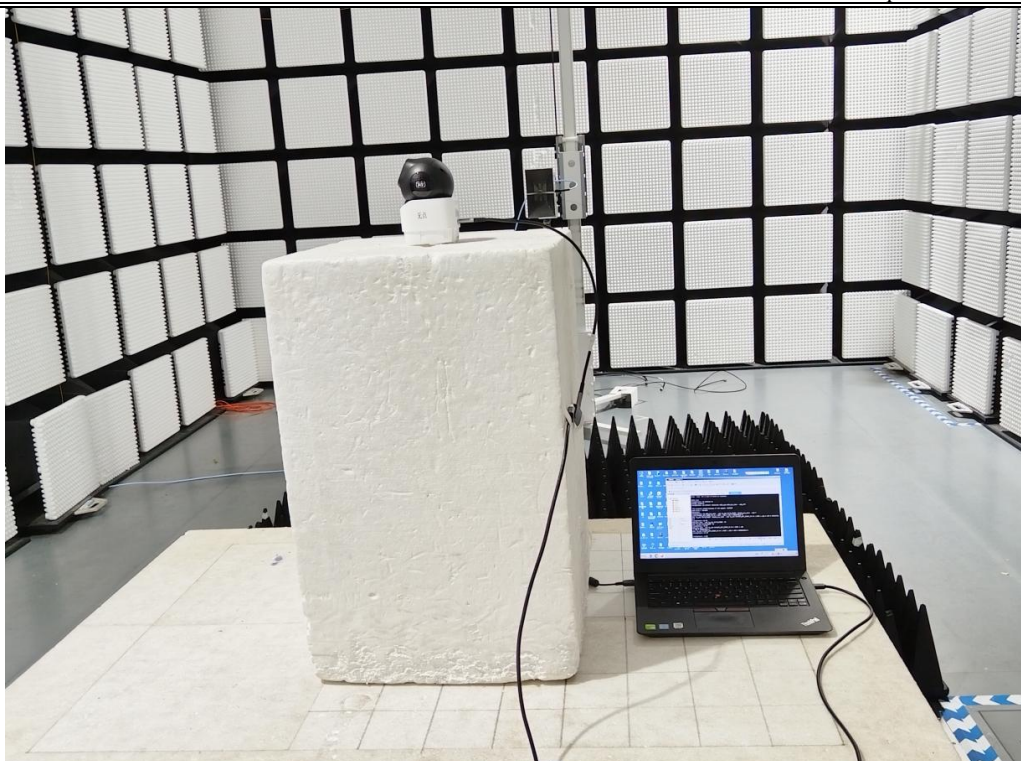
Fig. 3 Radiated emission setup photo(Above 1GHz)
