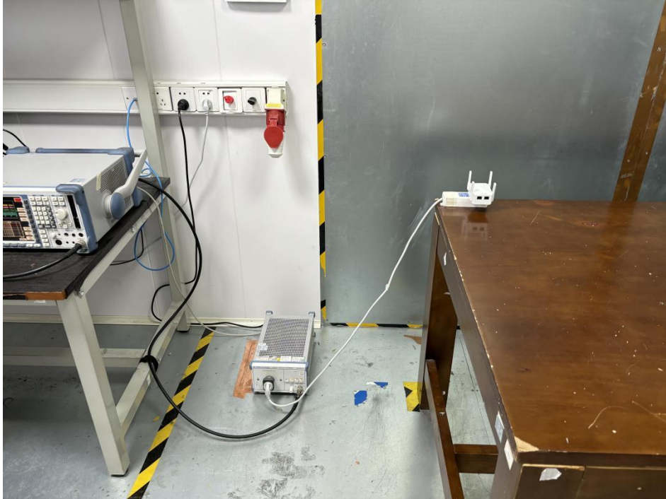
Conducted emissions at AC power line (150kHz-30MHz)
