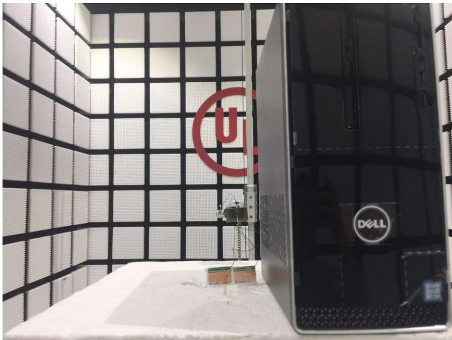
RADIATED RF MEASUREMENT POSITION (Z axis)
