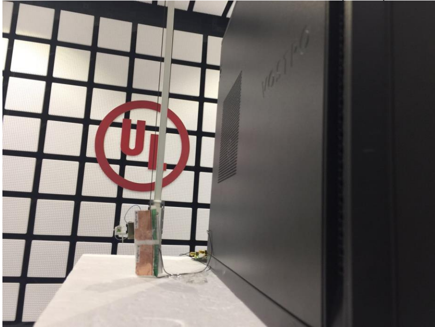
RADIATED RF MEASUREMENT POSITION (Z axis)
