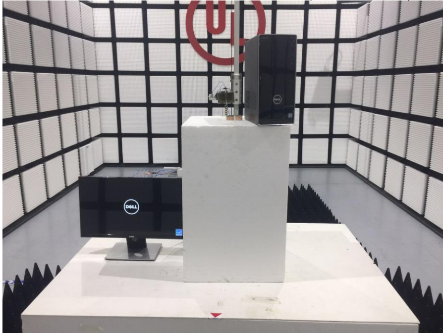
RADIATED RF MEASUREMENT SETUP DETAIL
