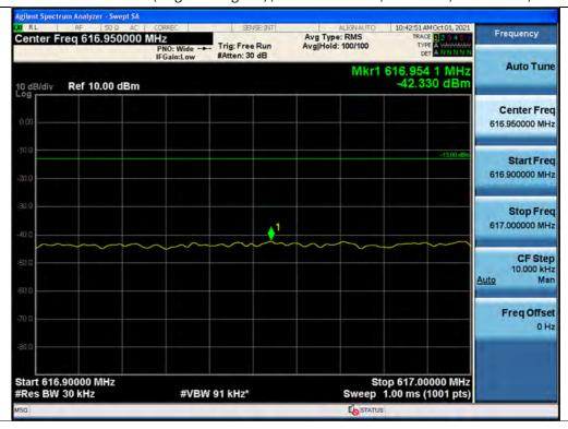
+3 dB above Out-of-band (single test signals) / 600 MHz Service / Downlink / LTE 20 MHz / Upper
