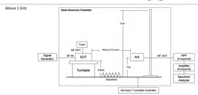
\*\* EUT position is adopted by placement of floor-standing refer to section 5.5.2.3.2 of ANSI C63.26-2015
