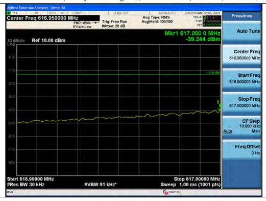
+3 dB above Out-of-band (two adjacent test signals) / 600 MHz Service / Downlink / LTE 5 MHz / Upper
