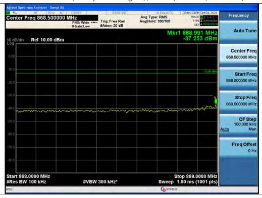
+3 dB above Out-of-band (two adjacent test signals) / Cellular / Downlink / LTE 10 MHz / Upper
