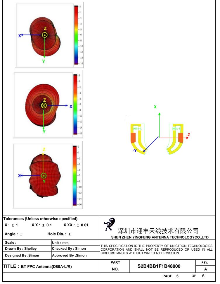
9-2.2D Gain complete machine (Radiation Pattern at 2450 MHz)
