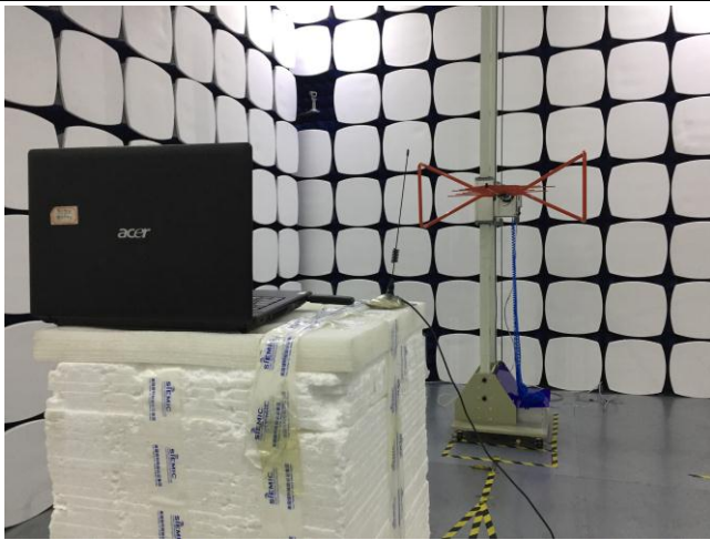
Radiated Spurious Emissions Test Setup Below 1GHz
