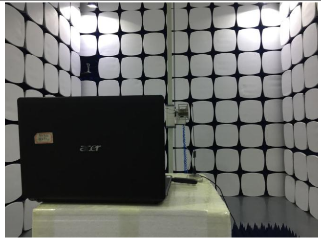
Radiated Spurious Emissions Test Setup Above 1GHz
