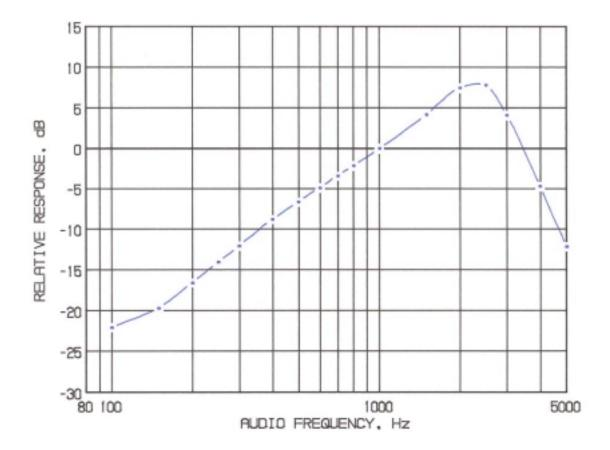
MODULATION FREQUENCY RESPONSE FCC ID: MMAG220
