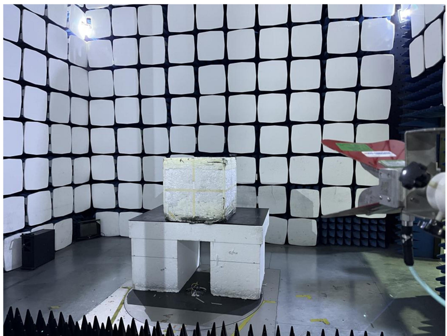
Radiation Emission Test Setup (1GHz to 18GHz)
