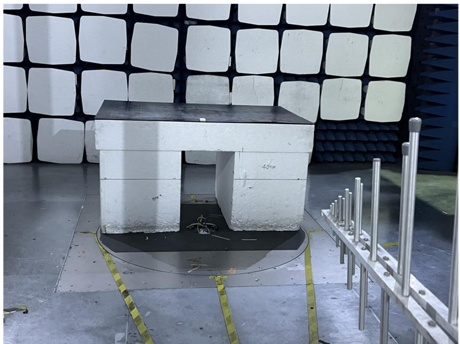
Radiation Emission Test Setup (30MHz to 1GHz)
