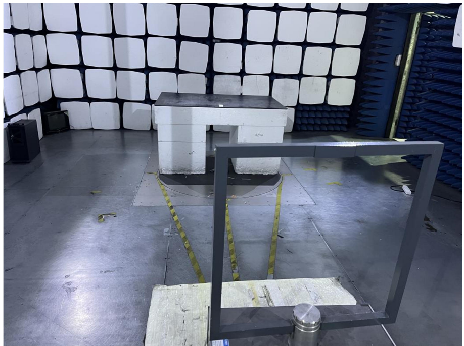
Radiation Emission Test Setup (Below 30MHz)
