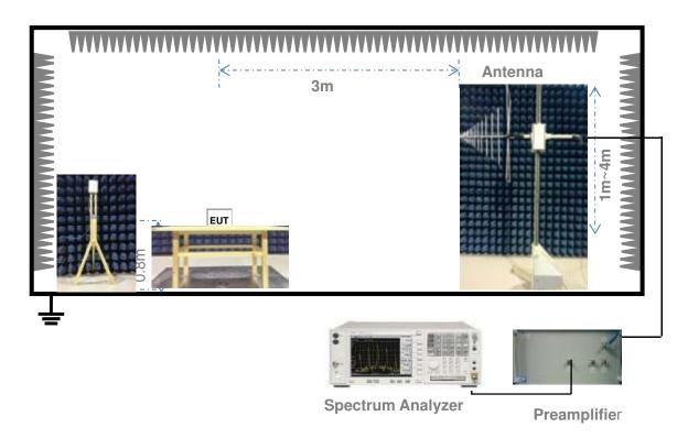
(For Radiated Emission Test (30 MHz-1 GHz))
