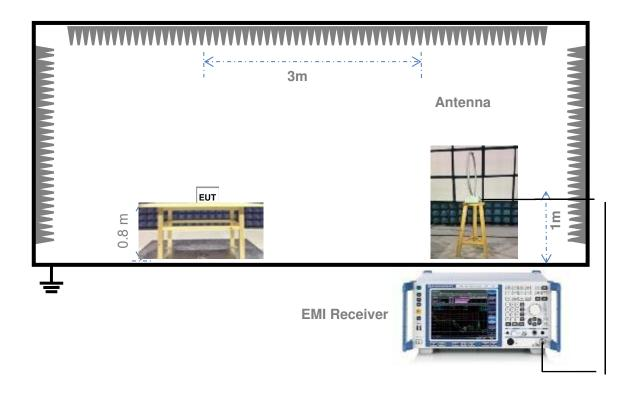
For Radiated Emission Test (Below 30 MHz))
