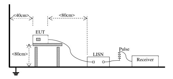
(For Conducted Emission, AC Ports Test)
