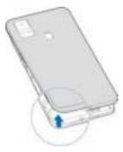
Install the nano-SIM card and the optional microSDXC card into the respective card slots.
