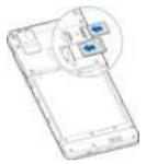
Insert the battery, making sure the connectors align. Gently push down on the battery until it clicks into place.
