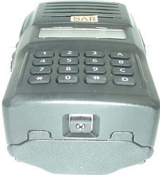
Bottom of DUT with 1150 mAh Li-ion Battery
