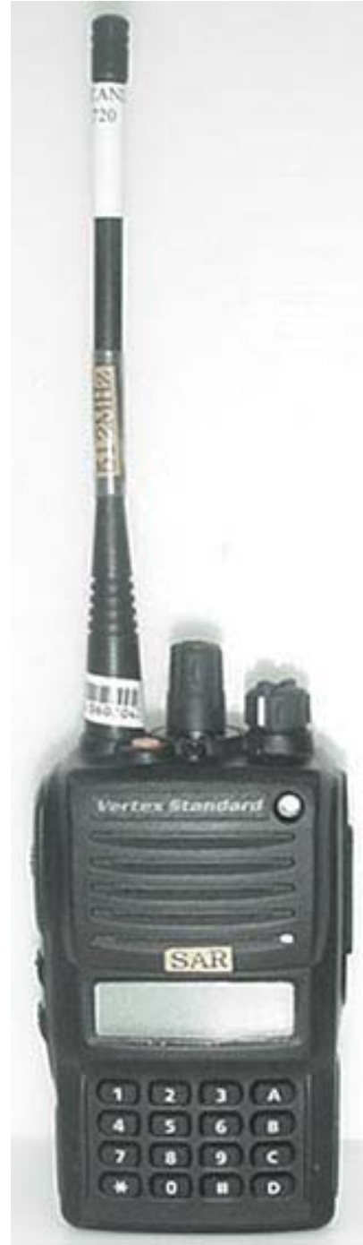
Front of DUT with Whip Antenna (512 MHz)
