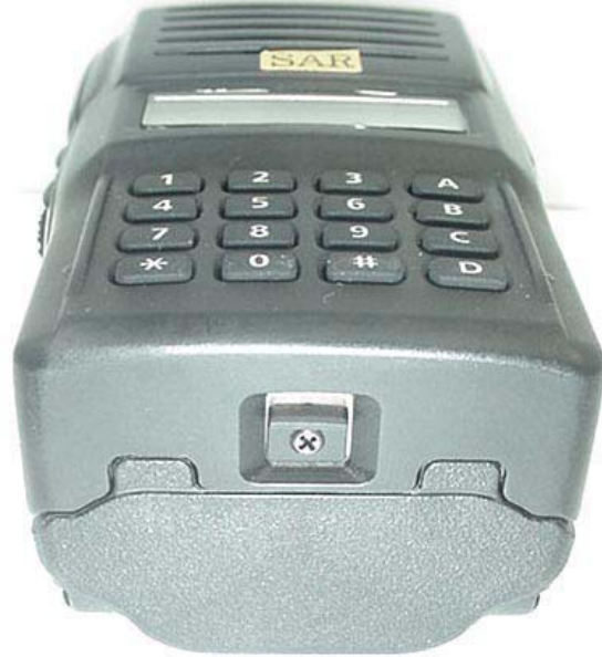
Bottom of DUT with 2000 mAh Li-ion Battery
