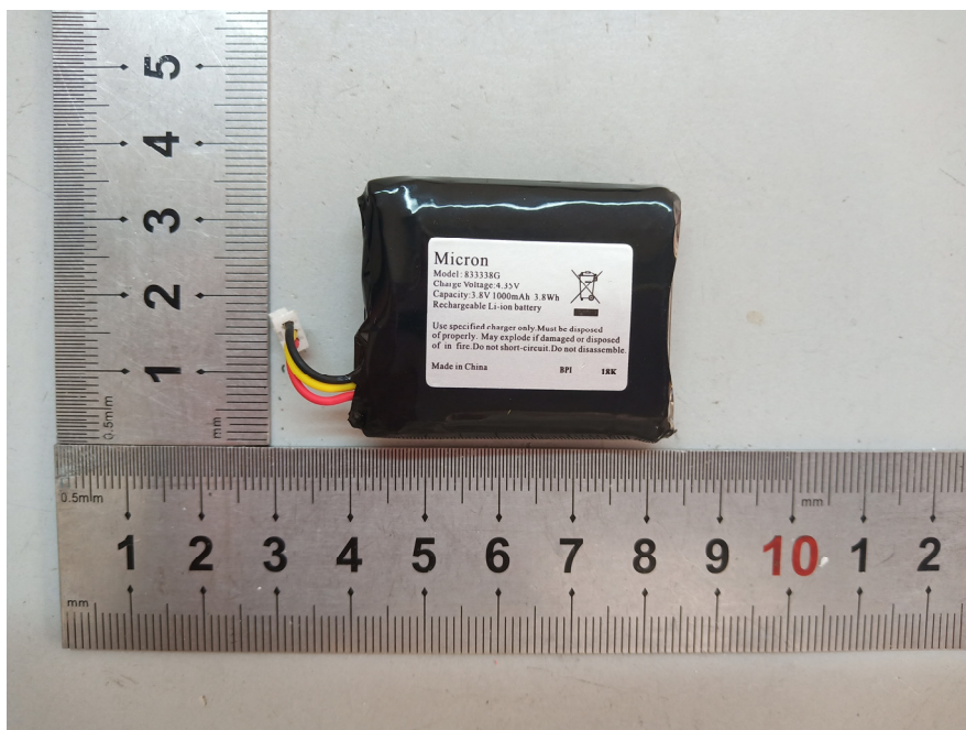
EUT –Battery View
