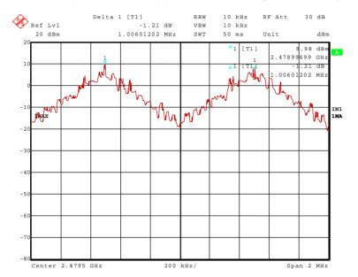
51145262.wmf: (channel separation at the upper end of the assigned frequency band):
