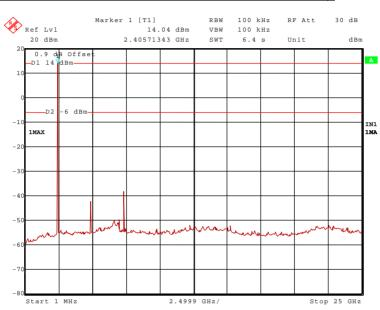
51145278.wmf (conducted emissions 1 MHz to 25 GHz, transmitter at 2441 MHz):
