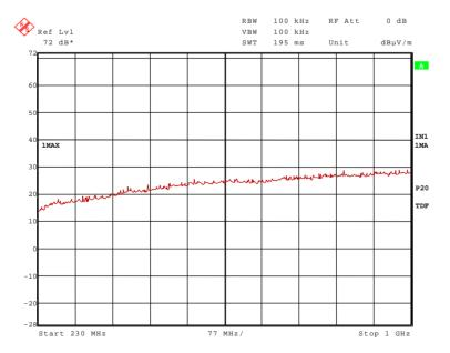
No significant frequencies above the noise floor of the system were found during the preliminary radiated emission test, so no measurements were carried out on the open area test site.
