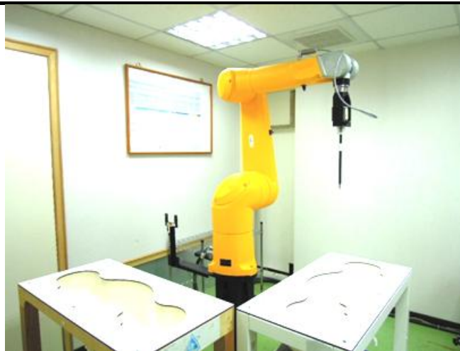
Fig-3.2 SPEAG DASY52 System
