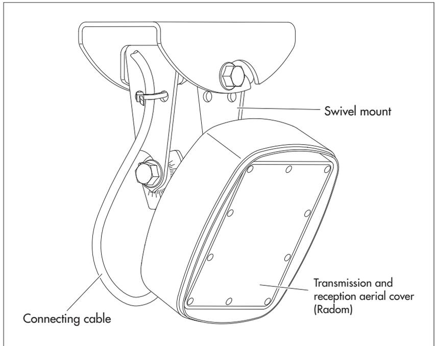
The cable length between the radar sensor and the data logger can be up to 1000 metres (depending on the wire cross-section used).
