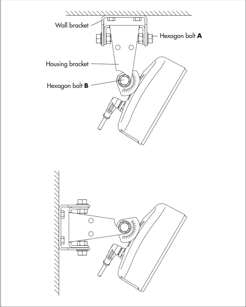
Fig. 11: Adjusting the sensor tilt angle ( $\alpha$ ) on the OTT SVR 100.
