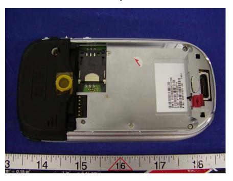
**EUT – PH10A/PH10B Chassis Cover Off View**
