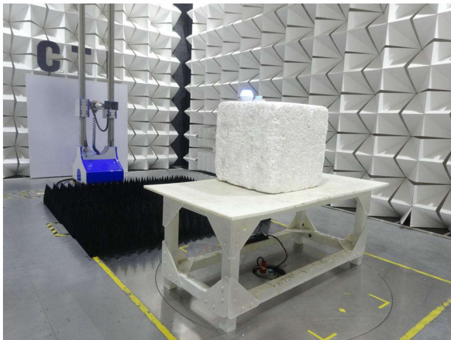
Radiated spurious emission Test Setup-3(Above 1GHz)
