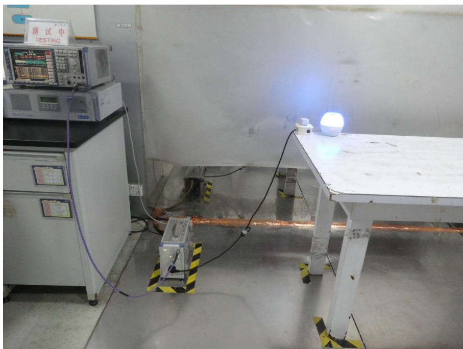
Conducted Emissions Test Setup
