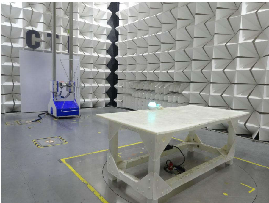
Radiated spurious emission Test Setup-2(30MHz-1GHz)
