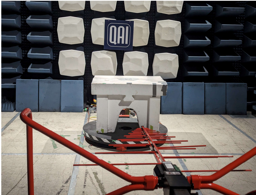
Figure 13: Radiated Emissions From 30 MHz to 1000 MHz Setup
