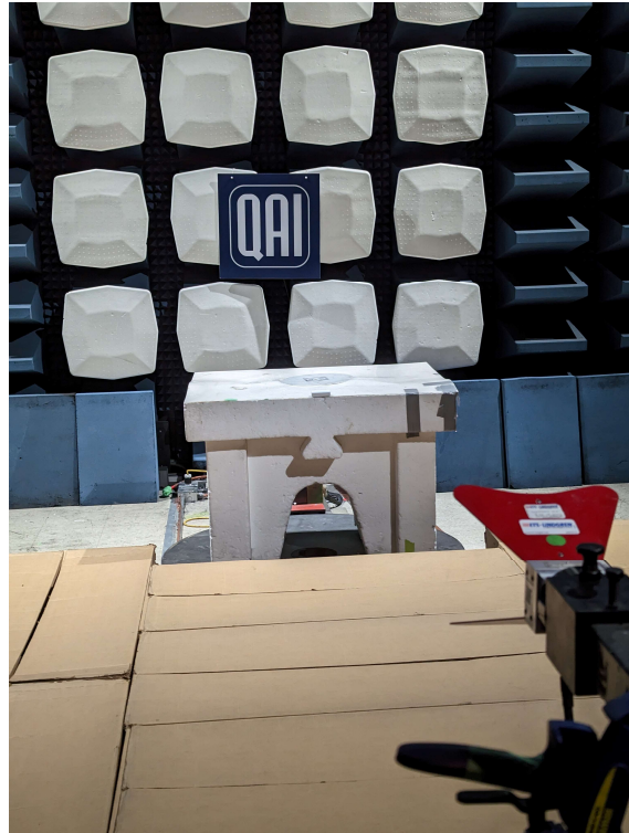
Figure 14: Radiated Emissions from 1 GHz to 6 GHz Setup
