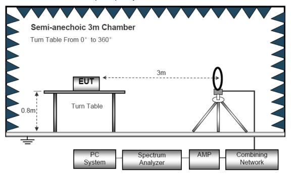
(B) Radiated Emission Test-Up Frequency 30MHz~1GHz
