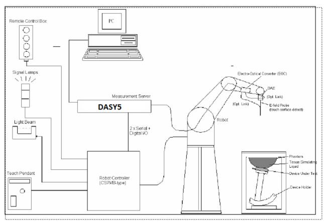
The DASY5 system for performing compliance tests consists of the following items:
