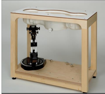
Picture C.8: SAM Twin Phantom
