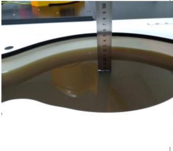
Liquid depth in the Body phantom
