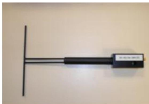
Figure 1 – Satimo COMOSAR Validation Dipole
