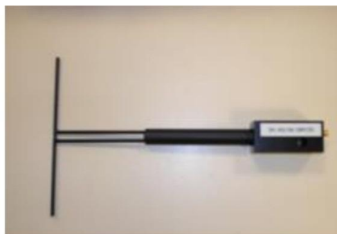
Figure 1 – Satimo COMOSAR Validation Dipole
