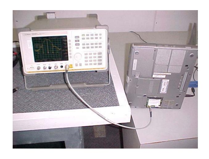
Conducted Emissions at Antenna Terminal Setup
