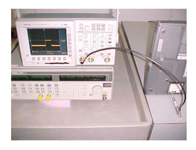
Maximum Peak Output Power Measurement Setup
