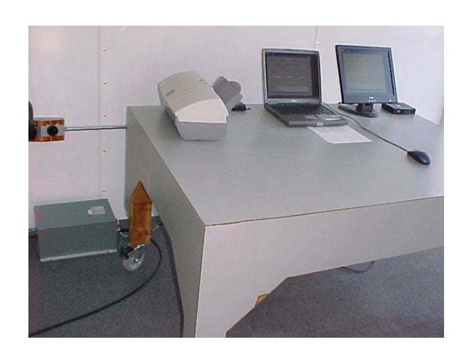
AC Conducted Emissions Measurement (Front View) Setup
