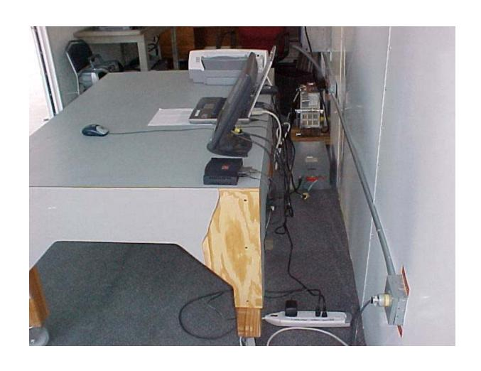
AC Conducted Emissions Measurement (Rear View) Setup
